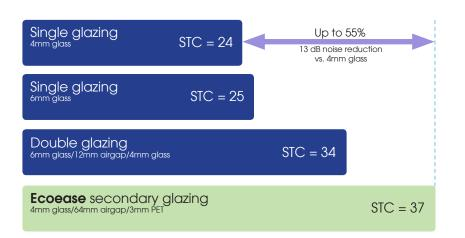
In the building industry, sound is measured in Sound Transmission Class (STC). An STC number is derived from sound attenuation values in decibels, tested at sixteen standard frequencies from 125 Hz to 4000 Hz. These decibel values are then averaged into one STC rating. An STC rating of 25 applied to a product will mean that an individual element reduces the sound passing through it by 25 decibels, averaged over the standard frequencies.
