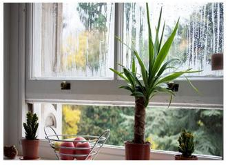
When the air travelling down the wall passes a cold window, conduction occurs causing the warm air to be cooled as it passes the cold pane of glass. This cooled air can then fall even faster and often causes a draught effect at the bottom of the windowsill. This results in cold spots being felt within the room.
