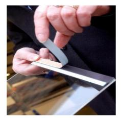
First take the steel tapes from the back of the edging as it is easier to cut with scissors. It needs to be cut square, not mitred.
