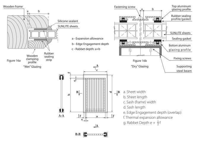
Figure 16 c. Schematic Sketch of Rebbet depth and Expansion Allowance. ("wet" and "dry" methods)
