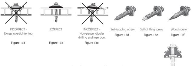
Figure 13. Typical Installation Screws & Obligatory Washers
