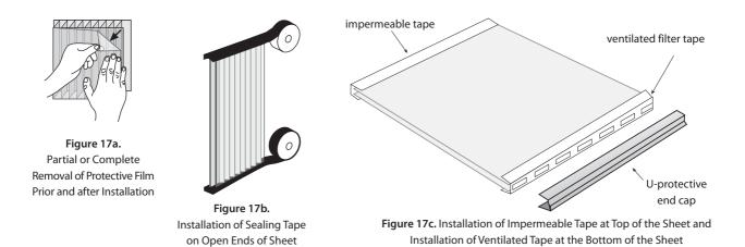
E. Ensure the use of the proper type of sealing tape according to the application used, verifying that the prepared sheets are mounted correctly. Please note: In case of curved installation, where both open ends are situated at the bottom - apply the ventilated tape on both ends. Take care to protect the sealing tapes at both ends from mechanical damage by inserting the edges into aluminium profiles, or cover them with polycarbonate U-shaped profiles (Fig-17c).
