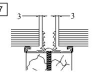
Put glazing material in place allowing for expansion:- 3mm per metre width and 3mm per metre length (at top end).
