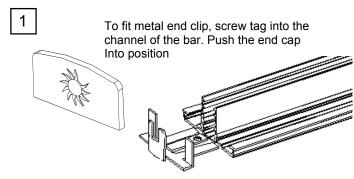
Screw bars to timber 100mm from each end and at equal intervals of 375mm.
