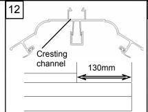
Remove cresting channel at both ends of ridge to allow for spider capping and water drainage.
