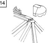
Slide cresting into cresting channel on and slide cresting and finial into top of ridge cap. Carefully cut the cresting channel to hold down spider spider top cap to fit over the hip bars. | cap.
