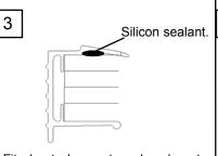
Fit sheet closure to polycarbonate or glass running a thin line of silicon sealant along the top inside face of the sheet closure.
