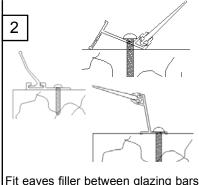
Fit eaves filler between glazing bars as required.
