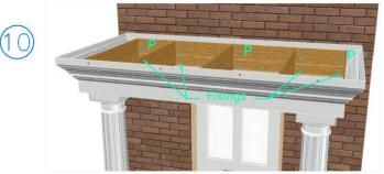
Once satisfied canopy is all level & even, put 3 fixings (1no into each brick course) adjacent to all baffles and at both ends of canopy - 7.5x100mm concrete fixings with oversize mudguard washers.
