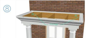
A third operative is to drill 6.5x120mm tight to both ends (centrally.) Fix using 7.5x100mm concrete fixings with oversize mudguard washers.
