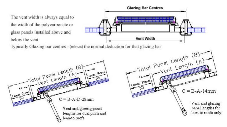
Vent panel length = vent length (A) – 135mm, Vent panel width = vent width – 135mm, (NB: if using glass then 24mm thick double glazed panels only)
